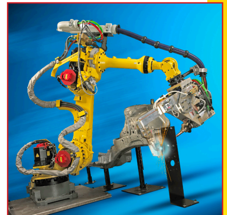
The R-1000iA/100F features factory installed process cable routing
